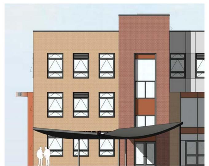
Detail Elevation showing brickwork and cladding colours
